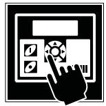
If no barcode is available, it is possible to enter the fusion parameters provided by the fitting manufacturer (like voltage and time) manually.
