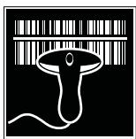
The barcode or QR code attached on most electro fusion fittings on the market contains all necessary data for processing them. After scanning with the scanner, this data is automatically transferred to the electrofusion unit and evaluated. The code essentially contains the following data: Manufacturer, type, diameter, fusion voltage, fusion time (with temperature correction, if applicable), resistance and resistance tolerance.
