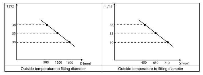
From a diameter of 630 mm (230 V devices) or 355 mm (110 V devices), longer cooling times of approx. 35 min must be ensured when the appliance is switched on (active cooling), otherwise the appliance will display the error message "Device too hot". In this case, it is necessary to let the electrofusion control unit cool down before putting it to use again.
