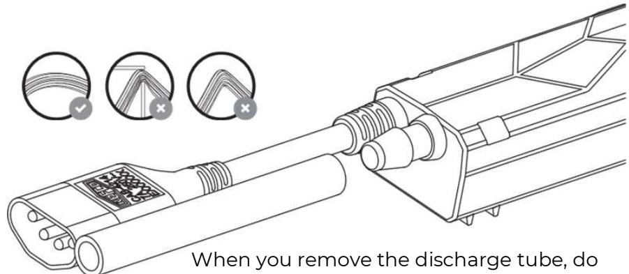
When you remove the discharge tube, do always use a knife cutting the tube. Too heavy force may destroy the pump.
