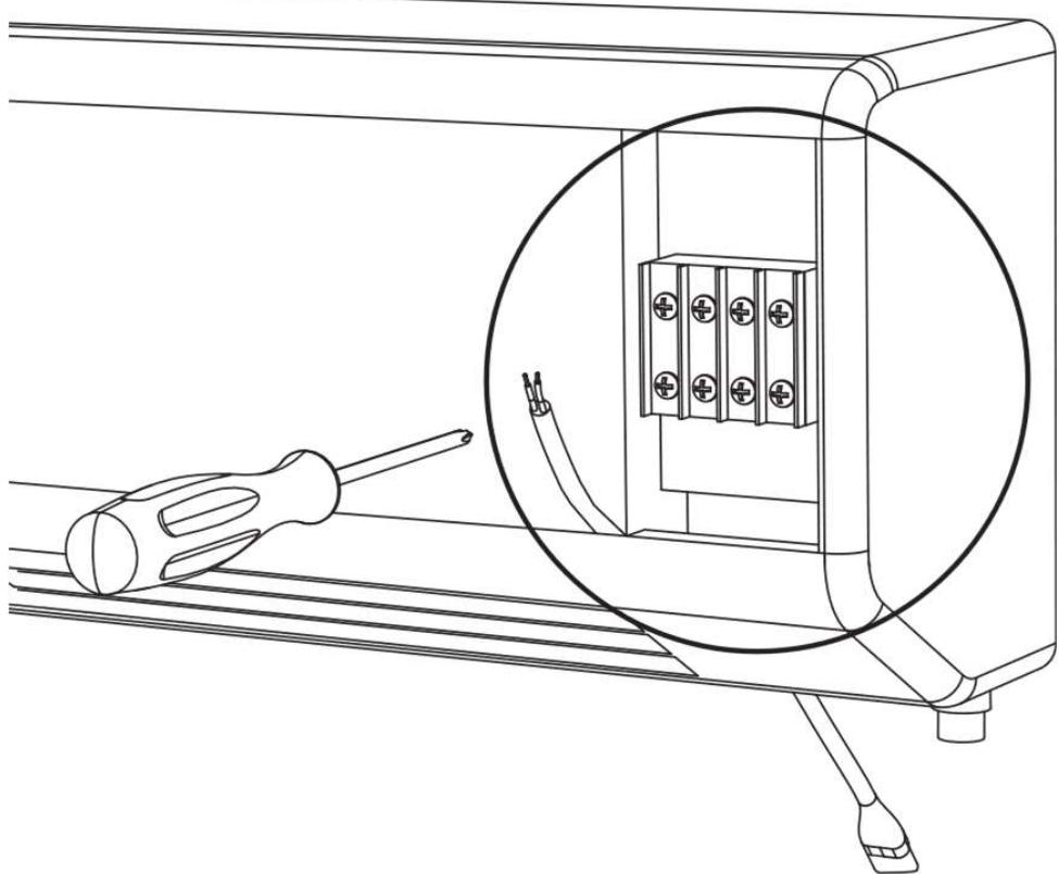
Optionally, the grey and violet wires can be connected to switch the power to the indoor unit. This will allow the pump to deactivate the unit in the event too much water is being generated for the pump to be able to handle.
