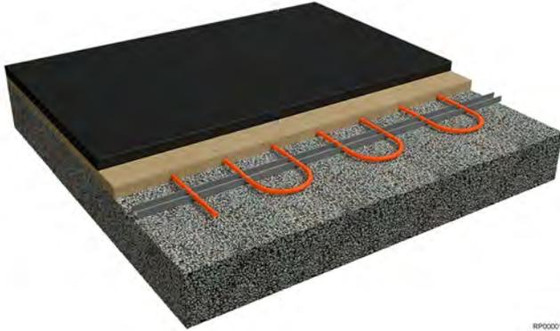
The image shows the basic installation of an asphalted structure with low wear. Mainly used for parking areas and truck loading areas with low traffic.
