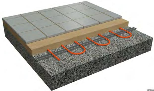
The image shows the installation of a Meltaway system under slab surfaced pavements and surfaces. The main usage is for pedestrian areas.
