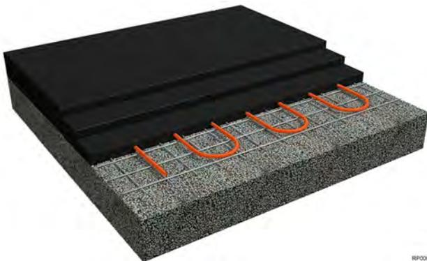
The image shows the installation of an asphalted structure with high wear. The main usage areas are parking area ramps, highly trafficked areas like roads and high truck traffic areas like the roads around logistic centers and so on.
