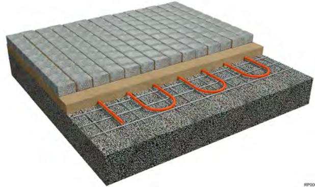
The image shows the installation of a Meltaway system under paving stones. Installation is done using Uponor industrial clamp tracks. The main usage for paving stone areas include pedestrian areas and roads.
