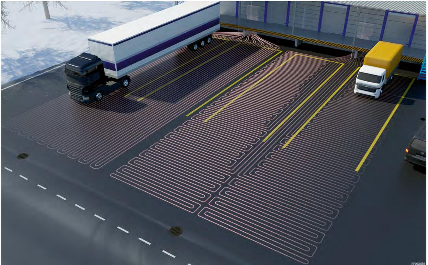
This illustration shows an example of a truck loading area with an Uponor Meltaway system design. There are four equal sized (160 m<sup>2</sup>) melting areas designed using two separate manifolds.
