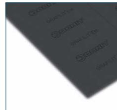
GRAFILIT® EM is an expanded graphite-based gasket material endowed with expanded stainless steel reinforcement for high operation pressures, including cycling loading. Uniform surface pressure distribution provides excellent thermomechanical properties and sealing characteristics, and increases blowout resistance. It is particularly suitable for high temperature applications in petrochemical industry and steam supply.
