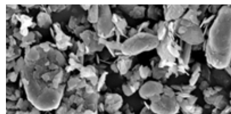
The main structure in Dixo® 7000 XP is a defined mix of graphite flakes and grains.
