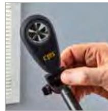
Thumbwheel for attaching/removing threaded universal end
