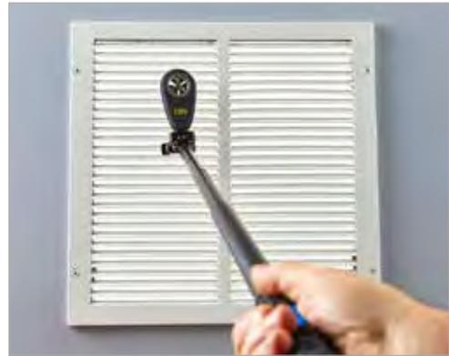
Attach the ABM-200, or TS-100 to the end of the EXP-64, to access hard-to-reach areas.
