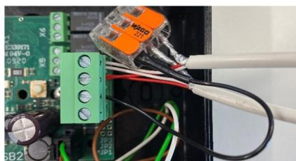
If the Analog Output is used, X1 4 and 5 have to be wired. The same ground potential for the AO and the connected device is required.
