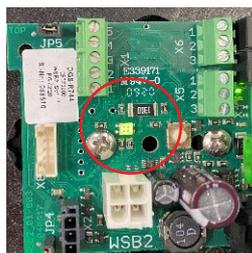
After a couple of minutes, the solid green LED means that the sensor is operating.
