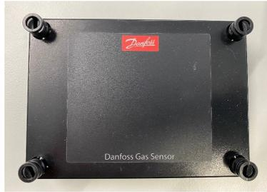
Once the 4 screws have been removed, you can access to the gas detector board.
