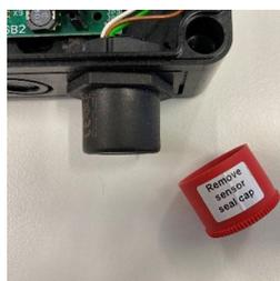
Remember to remove the sensor red cap protection, in order to make the sensor correctly operate.
