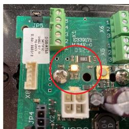
Once the power is provided you will see the yellow LED blinking, that means that the sensor is warning up.
