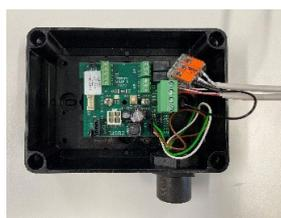
Make sure to not interrupt the shield when connecting A and B.
