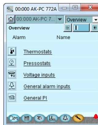
All the defined general functions are shown in overview display 2. In addition to always being shown in display 2, functions can be selected to be shown in display 1. Individual functions can be selected for display in display 1 via the "Show in overview display" setting.
