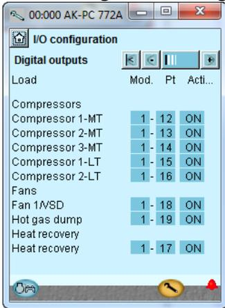
The setup of the digital outputs appears as it is supposed to according to the wiring made.
