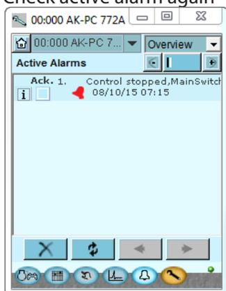
In our case an active alarm remains because the control has stopped. This alarm must be active when control has not started. We are now ready for the startup of control.
