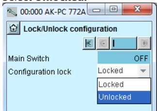
The controller can only be configured when it is unlocked.
