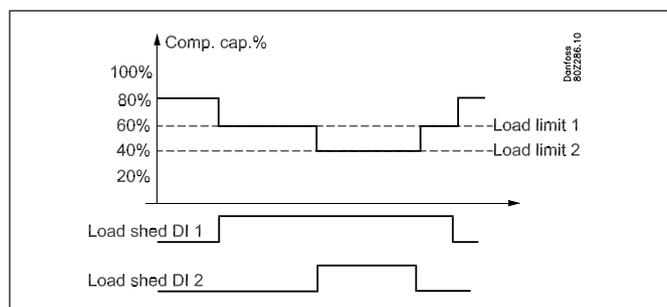
When both load-shedding signals are active, the lowest limit value for the capacity will be the one that is applicable.
