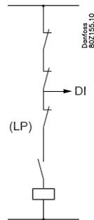
If a low-pressure switch is placed in the safety circuit it must be placed at the end of the circuit. It must not cut out the DI signals. (There is a risk that the regulation will become locked and that it will not start again). This also applies to the example below.
