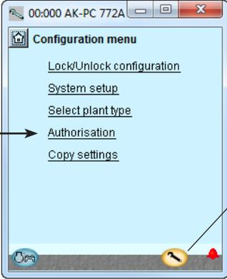
When the controller is supplied it has been set with standard authorization for different user interfaces. This setting should be changed and adapted to the plant. The changes can be made now or later.
