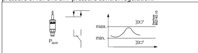
The pressure control can either use one of the sensors used by the control function (P<sub>o</sub>, P<sub>c</sub>) or an independent sensor (P<sub>aux1</sub>). Cutin and cutout limits are set for the pressure control. Coupling of the pressure control's output will be based on the actual pressure. Alarm limits can be set for low and high pressure, respectively, including separate alarm delays.
