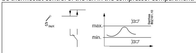
The thermostat can either use one of the sensors used by the regulation (S<sub>s</sub>, S<sub>d</sub>, S<sub>c3</sub>) or an independent sensor (S<sub>aux1</sub>). Cutin and cutout limits are set for the thermostat. Coupling of the thermostat's output will be based on the actual sensor temperature. Alarm limits can be set for low and high temperature, respectively, including separate alarm delays.
