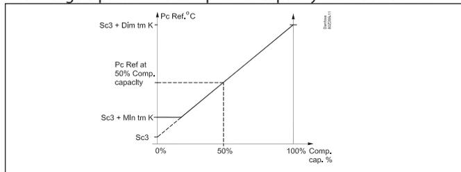
The minimum temperature difference (min tm) at low load should be set at approximately 2 K as this will eliminate the risk that all fans will be running when no compressors are running. Set the dimensioned difference (dim tm) at max. load (e.g. 3 K).
