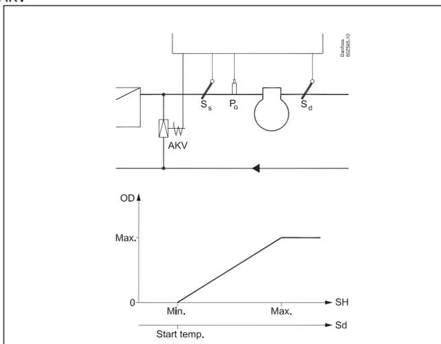
Four values are adjusted -- a start value for the  $S_d$  temperature, min. and max. values for overheating and a period time for the AKV valve.
