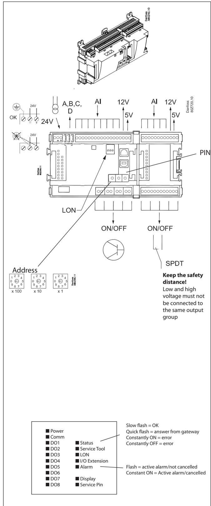
A small module (option board) can be placed on the bottom part of the controller. The module is described later in the document.
