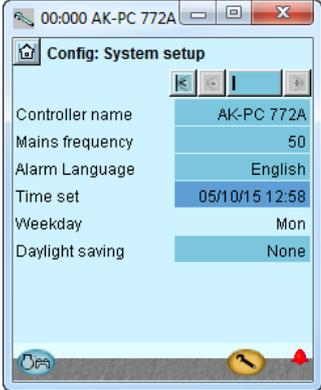
All settings can be changed by pressing in the blue field with the setting and then indicating the value of the required setting.
