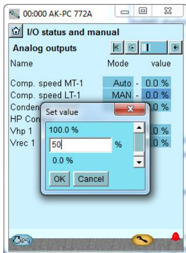
6. Put the control of the output voltage back to automatic
