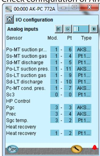
The setup of the analog inputs appears as it is supposed to according to the wiring made.
