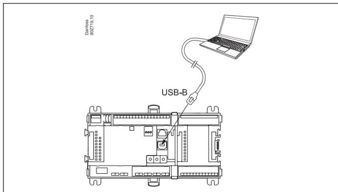
The controller must be switched on first and the LED "Status" must flash before the Service Tool program is started.
