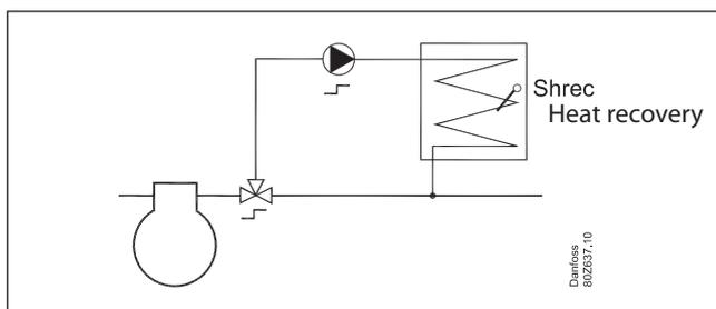
The heat recovery function can be used on the installation when you want to make use of warm gas for heating purposes. When the function is activated the reference for the condenser temperature will be raised to a set value. If the controller must also activate a pump and/or a valve, a relay must be selected for the function.
