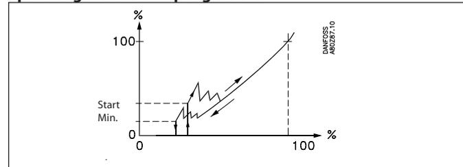
The controller starts the frequency converter and the first fan when the capacity requirement corresponds to the set starting speed.
