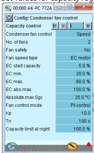
In our example the condenser pressure is controlled on the basis of the Sgc and from Sc3 (floating reference).
