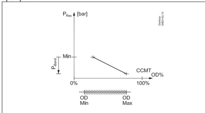
The settings OD Min. and OD max. are adjusted as % of the degree of opening.
