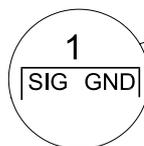
At the bottom the signal input is the right of the two terminals.
