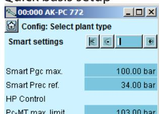
In our example, the controller must regulate a Booster System, High Pressure Control
