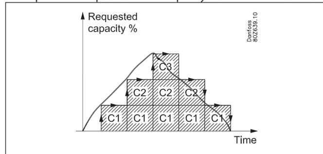
Cut-out of the last compressor stage:
