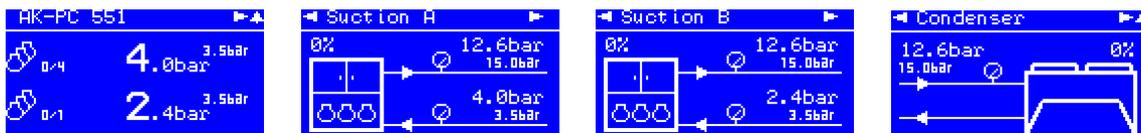
Each of the four rows above is continued with three additional displays. The arrow in the top corner of the display shows the way to the next display in the same area of operation. By clicking the right arrow you can see these three displays:
