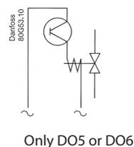
The capacity is divided into period times as "PWM period time". 100% capacity is delivered when cooling takes place for the whole period. An off time is required by the bypass valve within the period and an on time is also permitted. There is "no cooling" when the valve is on.
