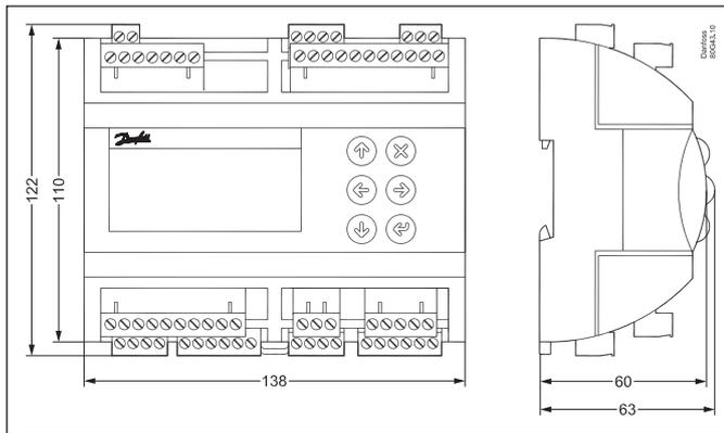
For DIN rail mounting only (IP 20)
