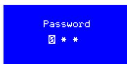
The default password upon delivery is 300. Use the arrow keys to set the password. End by pressing "Enter"  $\leftarrow$
