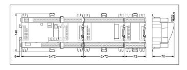
Example continued: Controller module + 1 extension modules in 100-series = 224 + 72 = 296 mm.
