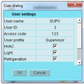
This is where you can select the supervisor for the specific system and a corresponding access code for this person.
