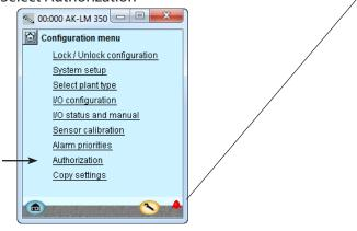
When the controller is supplied it has been set to show the default authorization for the different user interfaces. This setting should be changed and adapted to the plant. The changes can be made now or later
