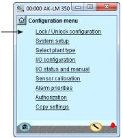
Select Configuration lock Press the blue field with the text
