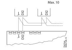
The following controllers can be connected up in this way: EKC 204A, AK-CC 210, AK-CC 250, AK-CC 450, AK-CC 550\_
