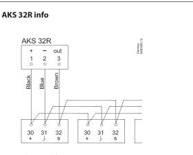
The signal from one pressure transmitter can be received by up to ten controllers. There cannot be a significant drop in pressure between the pressure transmitter's position in the suction line and the S2 temperature in the individual evaporators.
