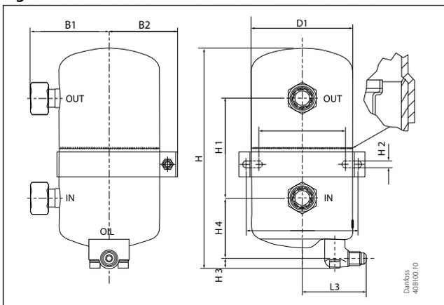
Figure 3: OUB 1/OUB 4 (flare & solder connection)
