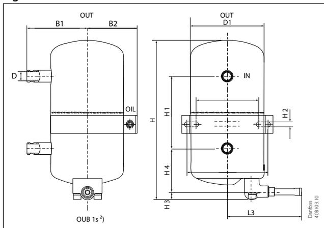
2) OUB 1s 6 mm ODF solder connection to oil return line.
