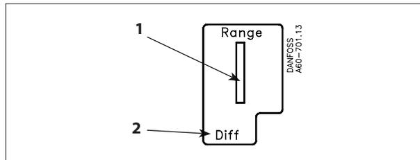
1. Adjust range spindle to desired LOW SET POINT (LSP)
