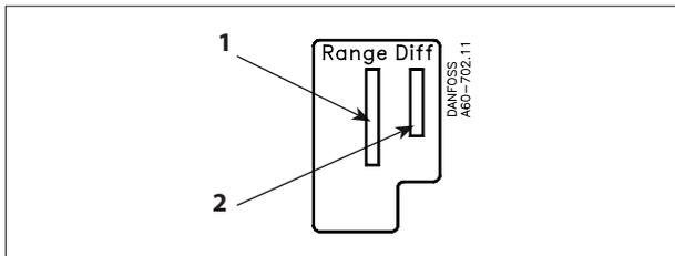
1. Adjust range spindle to desired HIGH SET POINT (HSP)
