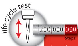
In accordance with the CAREL development procedure, E2V-CW has also undergone lifetime testing to confirm reliable operation even after 1.2 billion steps completed in the most demanding working conditions.
