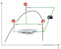
The reliability of CAREL valves for  $CO_2$  is also guaranteed by extensive, rigorous development tests: > 1.2 billion steps, according to the AHRI standard corresponding to more than 10 years' operation in real applications.
