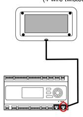
Connection for POL871.72 Cable length Cable type Cable with RJ45 plugs on both sides 1.5 m Separated Cat-5 Ethernet cable with two RJ45-plugs (8-wire twisted pair)
