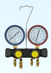
ITE presents a new 4-way manifold without sight glass. New style composition disc gate valves ensure leak tight deep vacuum and higher pressure operation. When fully opened the valves have no obstruction in the flow path, resulting in very low flow resistance. This 4-way manifold can be used with refrigerants such as R410A, R32 and CO2 in subcritical applications.
