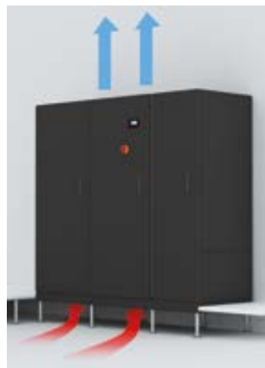
Version with air intake from the bottom, stand for raised floor, blind front panel and upflow air supply.
