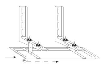
B- Fix the hooking brackets to the brackets (1) and insert the screws at the side (2).
