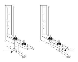
C- Insert the water collection tray into the prepared tracks.
