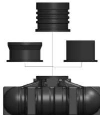
Clean the contact surface of the extension neck, carefully position it in the centre and set it down on the tank. Avoid moving the extension neck to the side once it is standing on the tank!
