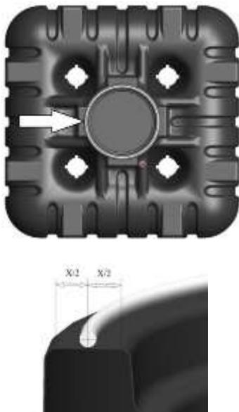
Clean and place a single string of the sealant/adhesive provided around the neck of the tank in the middle of the area.
