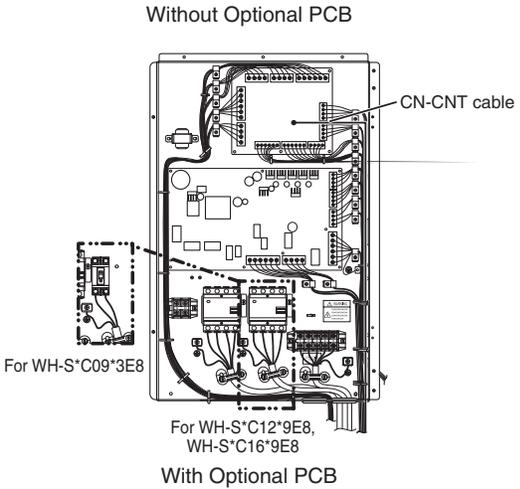
2. **Insert a flat head screwdriver into the slot on the top of the adaptor and remove the cover. Connect the other end of the CN-CNT cable connector to the connector inside the adaptor.**
