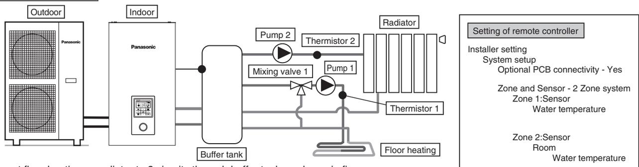
Connect floor heating or radiator to 2 circuits through buffer tank as shown in figure.
