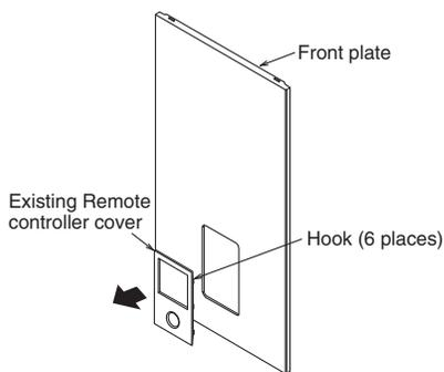
2. Press from front to fix the Remote controller cover ⑥ on the front plate.
