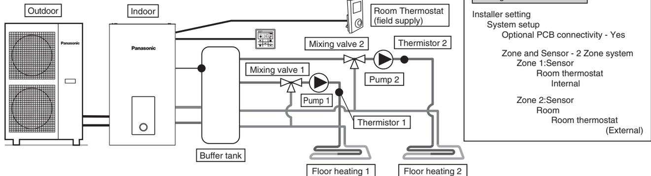
Connect floor heating to 2 circuits through buffer tank as shown in the figure.
