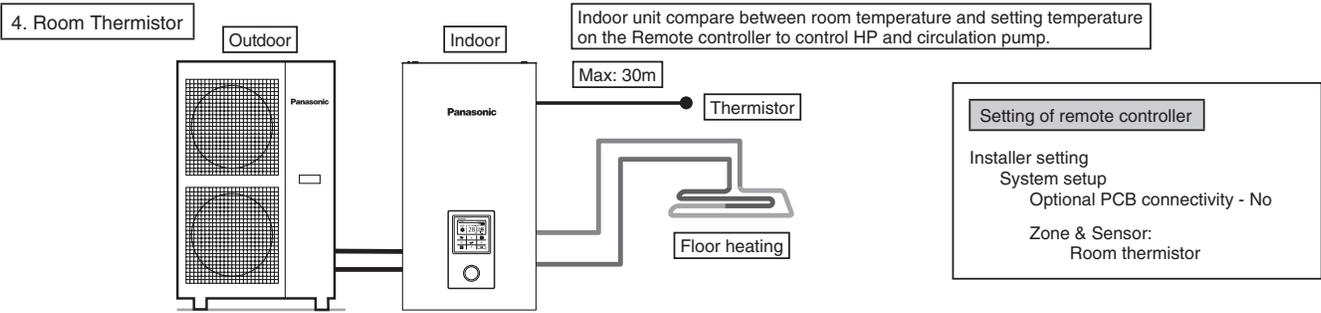
Connect floor heating or radiator directly to indoor unit.
