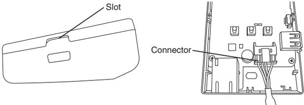
3. **On the wall near the Indoor Unit, attach the adaptor by screwing screws through the holes in the back cover.**
